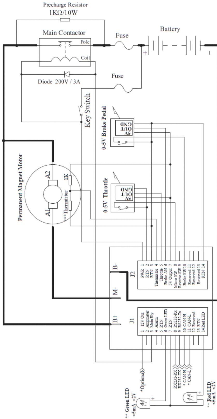
NOTE: 0-5K potentiometer can be used as throttle signal. Wire 5V and RTN to two end terminals, and wiper will output 0-5V signal.
