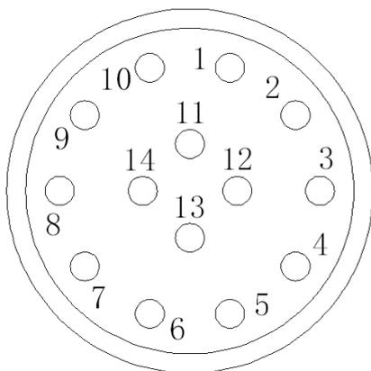
**Figure9:** The connecting diagram of **J1** and **J2**
