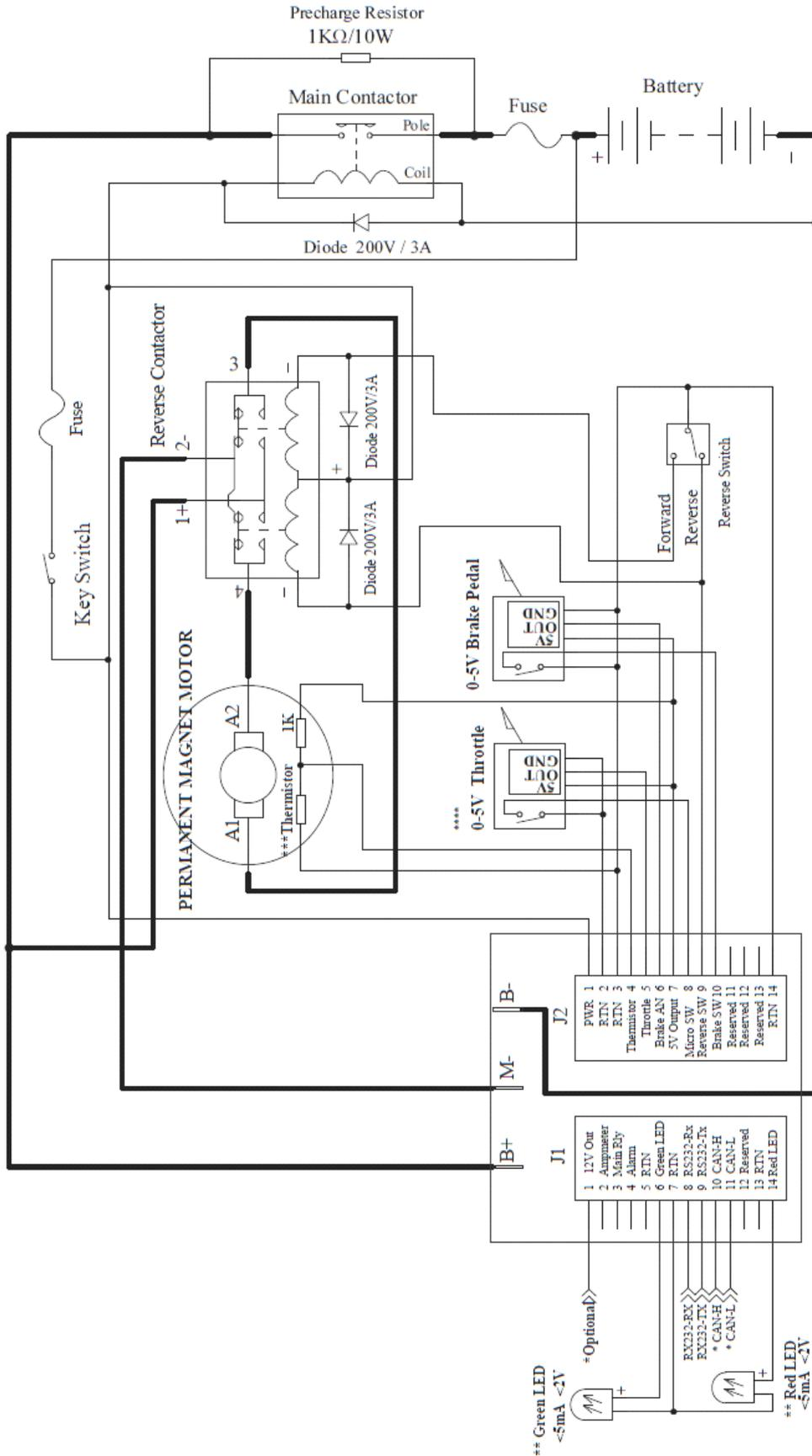
NOTE: Potentialmeter can be used to output 0-5V. Wire 5V and RTN to two end terminals, and wiper will output 0-5V signal. Please securely wire B- before any other wiring. Never put contactor or break on B-.
