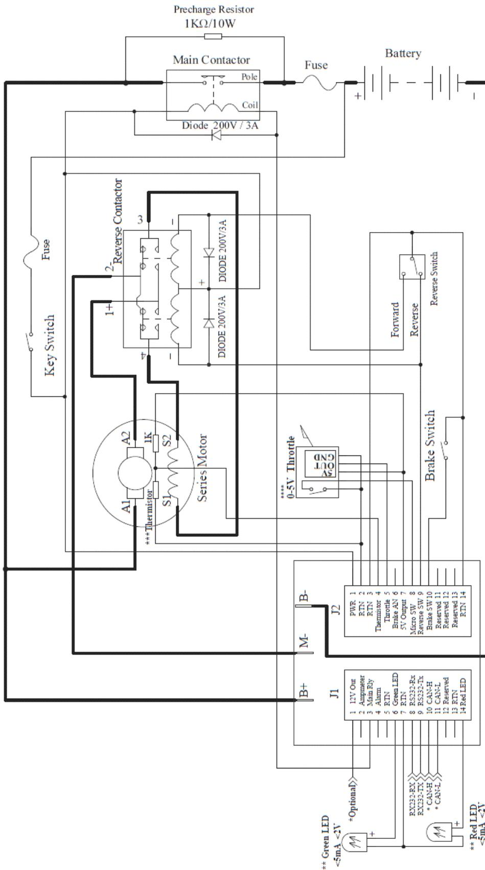
NOTE: 0-5K potentiometer can be used as throttle signal. Wire 5V and RTN to two end terminals, and wiper will output 0-5V signal.
