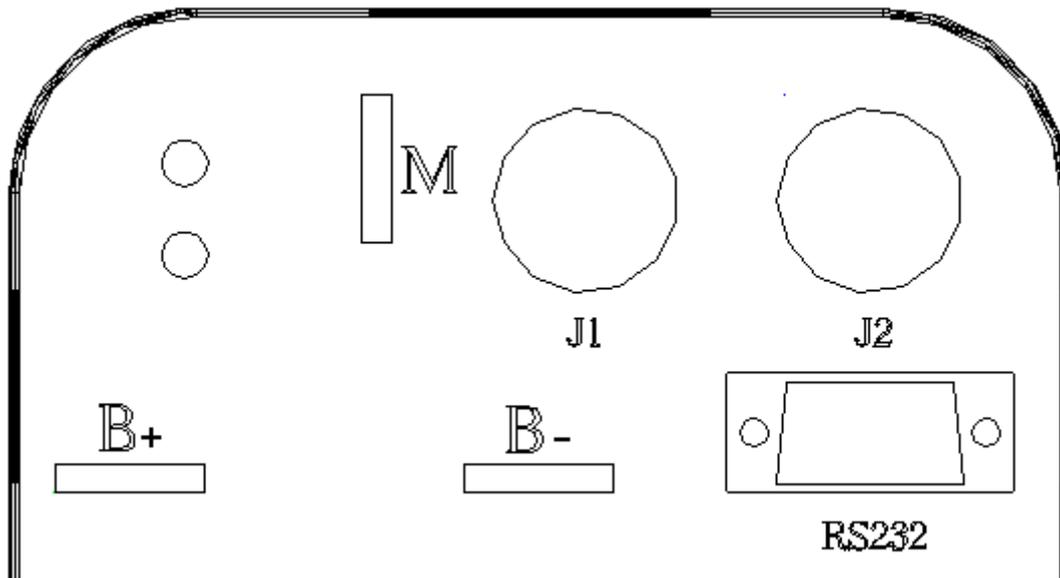
**Figure 2:** Front panel of KDZ motor controller
